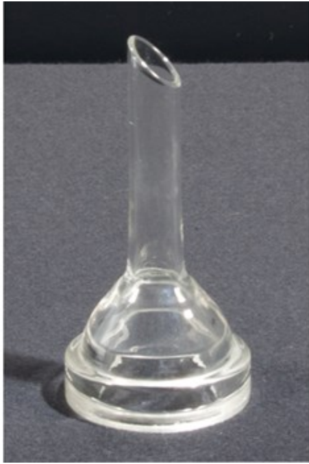
Filter funnel w/ porous plate for filtration set
