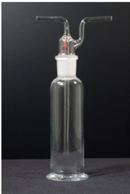
Gas wash bottle w/o porous plate 250 ml
