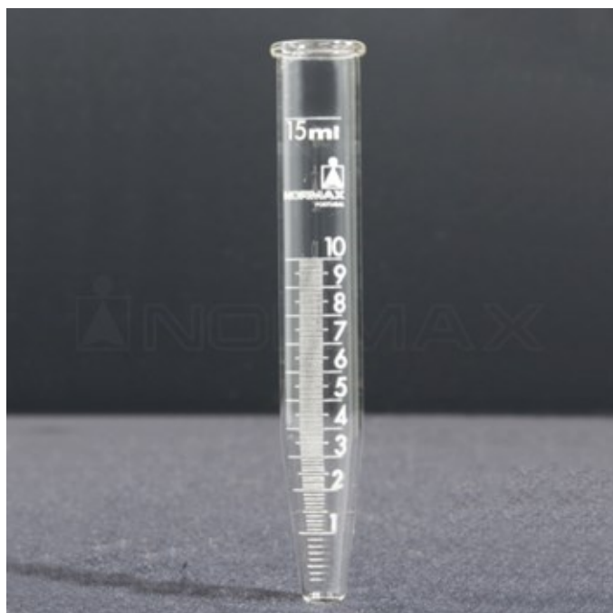
Centrifuge tube conical bottom neutral glass graduated 16x110 mm
