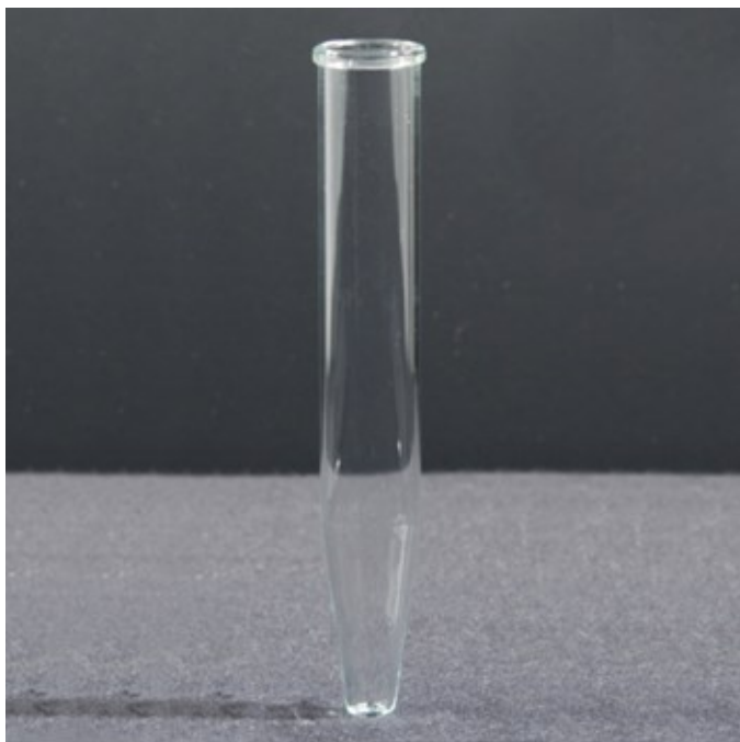
Centrifuge tube conical bottom, plain, neutral glass 17x115 mm
