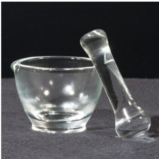
Glass mortar with spout and pestle, Ø80 mm, 100 ml
